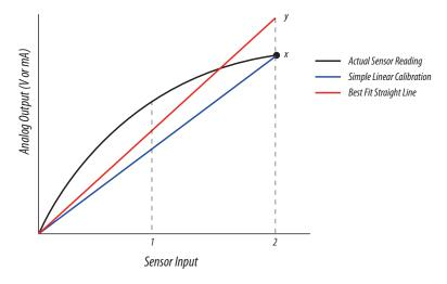
To calibrate a sensor using the BFSL, adjust the panel so that when the sensor reading is at full scale (x), the output will be set to the value at point (y). This will halve the overall linear error.
